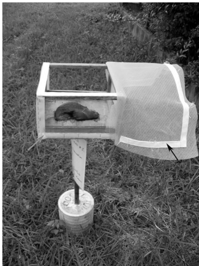
FIG. 2—An open cage exposing the bait (Phase I). Strips of hook (gray arrow) and loop (black arrow) of Velcro fasten while closing the cage.
